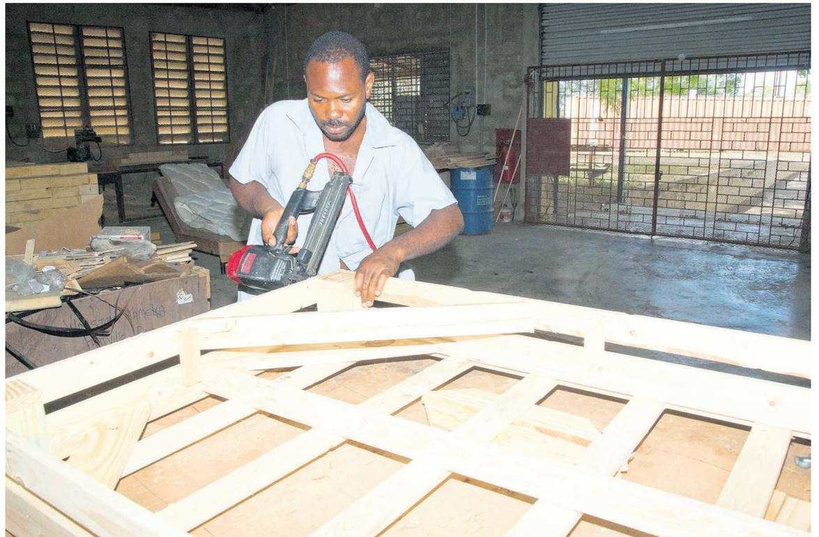
A workman at the manufacturing plant constructing the base of a bed at Morgan's Group.
